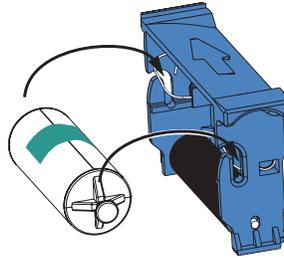
2. Peel the protective wrapper from the Adhesive Roller.
