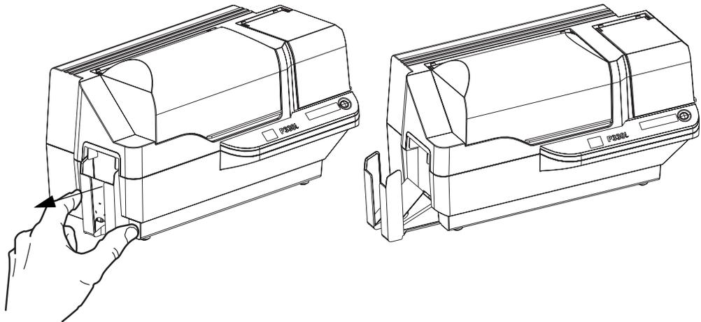
2. When not using the printer, slide the card output hopper back into its closed position to protect the printer from dust and protect the output hopper from damage.
