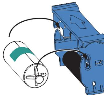
5. Peel protective wrapper from the cleaning roller by gently pulling on the tape.
