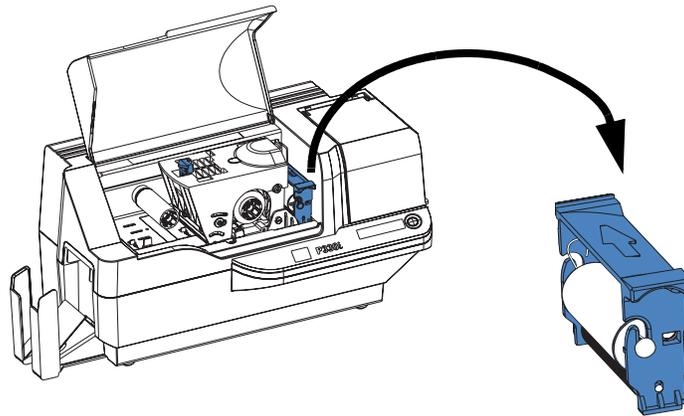
3. Remove the cleaning roller from the Card Cleaning Cartridge and discard.
