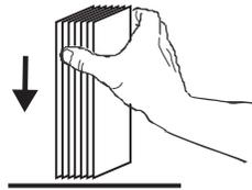
4. Push the stack back and forth to an angle of about 45° from vertical, so as to separate all of the cards.
